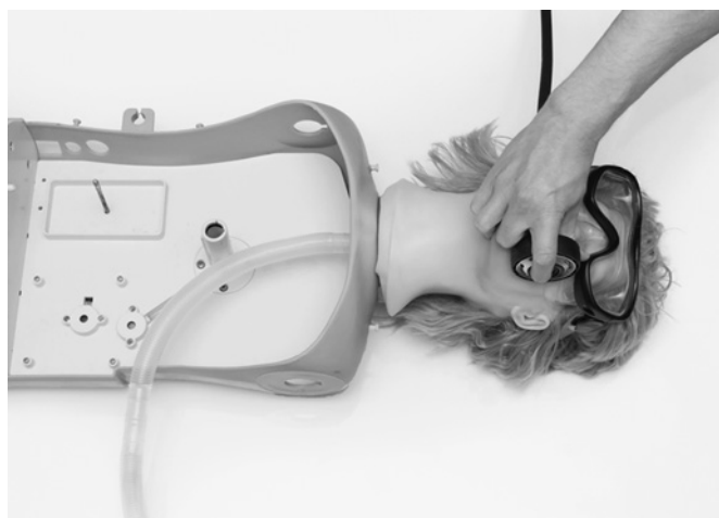
Figure 1 Test setting for the assessment of peak pressures. The hose attached to the upper airways of the manikin is directly connected to the Primus ventilator for pressure measurement. The one-handed technique is used to operate the SCUBA regulator.
